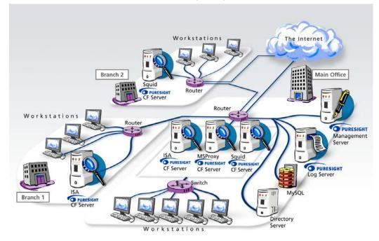
This example shows PureSight deployed in a network with a headquarters and two remote branch offices.
